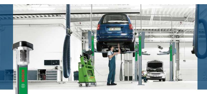
Hardly any other equipment in the workshop is used as often as the lifts. For inspections of the vehicle's underbody, brake repair and a lot more. The lift moves the vehicle to an ergonomic height, thus making repairs easier to carry out.
