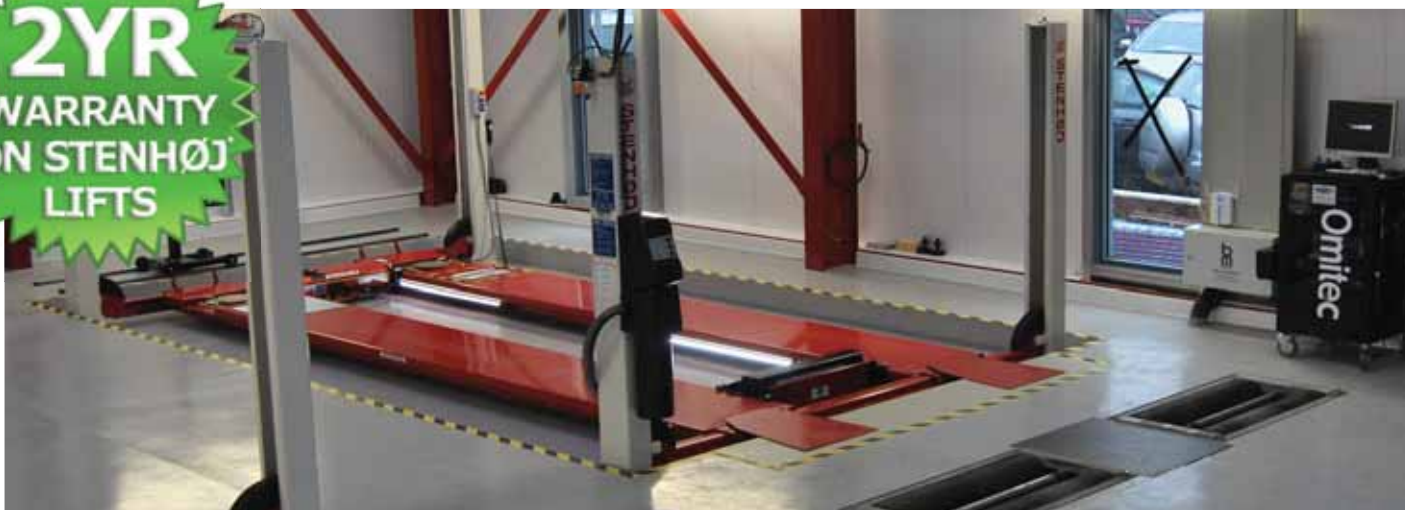
ATL Bay with Stenhøj 4 tonne lift (model 4026-47)
