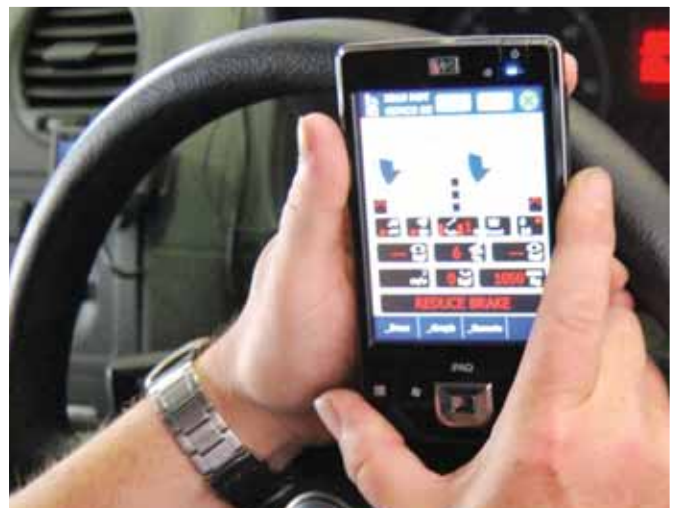
PDA for operation of roller brake tester
