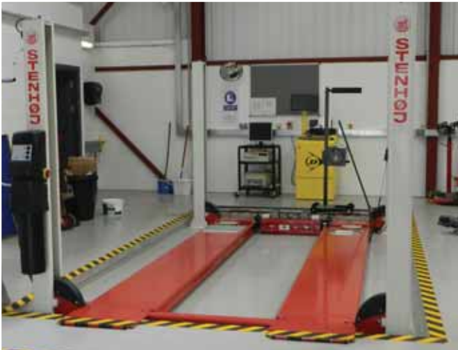
Stenhøj ATL Lift in 130mm purpose built recess
