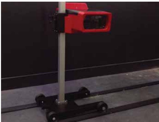
GEMCO Litecheck4 double laser with 3m of rails
