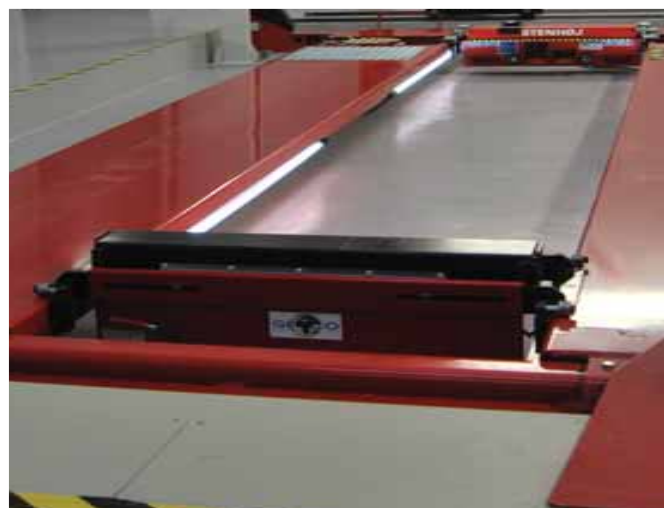
Jacking beams fitted to Stenhøj ATL lift
