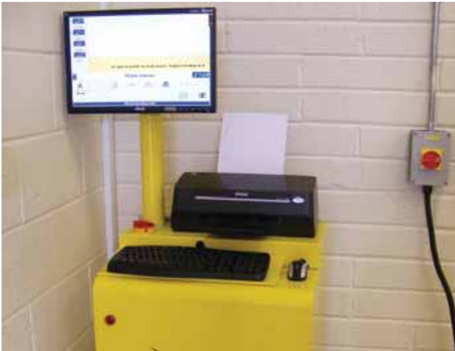
PC with ATL Software on DUNLOP ATL Brake Tester
