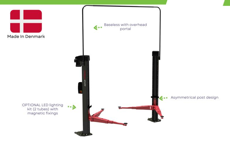
The AUTOPSTENHOJ 099351 Maestro 2.32 F NxT two post lift features asymmetrical posts which are very stable (welded not bent). Quality 3 phase motors power the screw and nut system contained within each post. An internal arm locking system on the arms ensures that 360 degree engagement is achieved.
