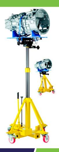
The VTJ2000 vertical transmission jack has been specially designed to assist the removal of gearboxes and transmission parts safely by 1 technician, with a 2-way tilt-and-turn adjustable adaptor, giving precise positioning of the load.
