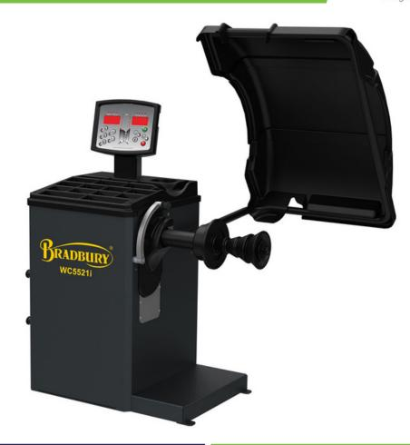
The Bradbury WC5521i Advanced Electronic Wheel Balancer features advanced Italian software with 7 different ALU modes. The machine has a hidden (split) weight feature, which means weights can be hidden behind the wheel spokes.
