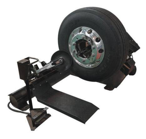
The Dunlop DTM588 is a very popular commercial vehicle tyre changing machine for wheels up to 59" diameter. The combination of heavy duty design and robust single-piece frame give this tyre changer a powerful but stable operation.
